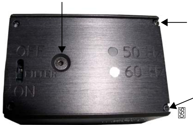
Figure 4.4n Unscrew These TUNA Screws to Remove the Top Panel
