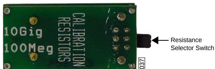
Figure 5.7a Test Resistor supplied with Extended TUNA Sensor
